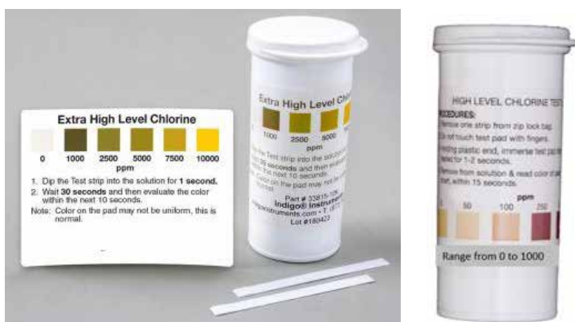
Fig 6.7 Extra high level strips (test concentration from 0 to 10,000) to check the original concentration of hypochlorite solution and high level strips (test concentration from 0 to 1000 ppm) to check the concentration of hypochlorite solution after dilution has been made before use
